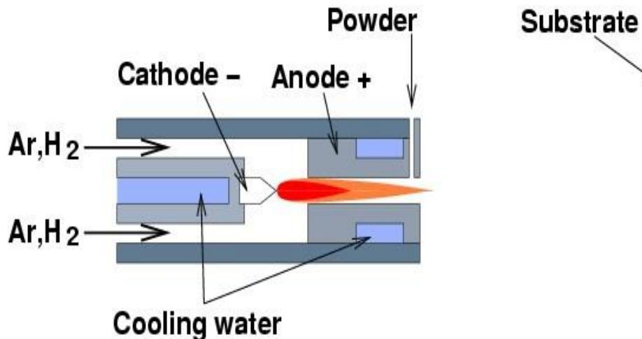
The scheme of formation of quality of coatings in the process of plasma spraying
