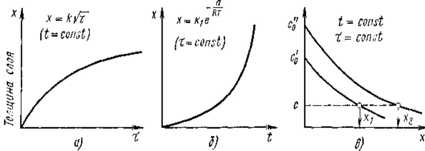
Chemical-thermal treatment (HTO) - the saturation of the surface of the metal or an alloy of one or more elements by its diffusion in the atomic state of the environment at a high temperature.
