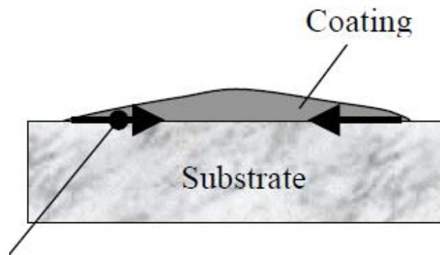
Tensile force applied by substrate due to coating particle shrinkage.
