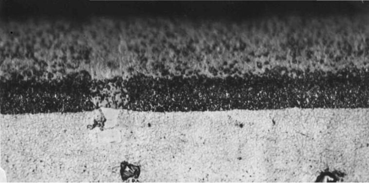
Aluminizing - saturation aluminum surface at temperatures in the 700-1100 ° C saturating respective environments.
