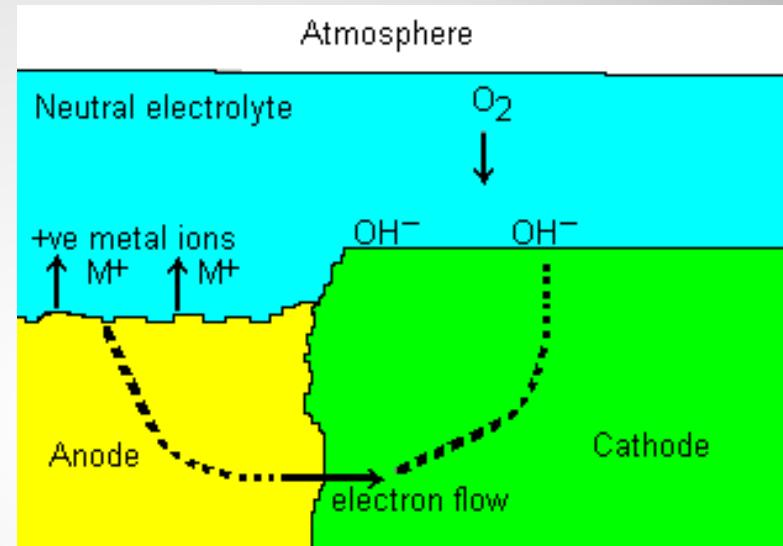
The surface of the metallic article may comprise a plurality of galvanic couples (anode-cathode).
