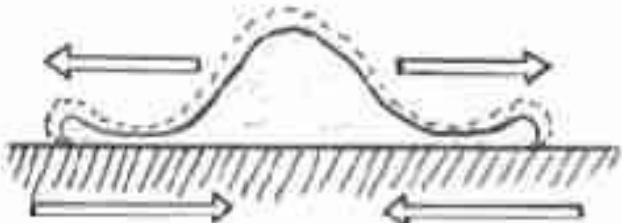
Compressive force applied to substrate by coating particle
