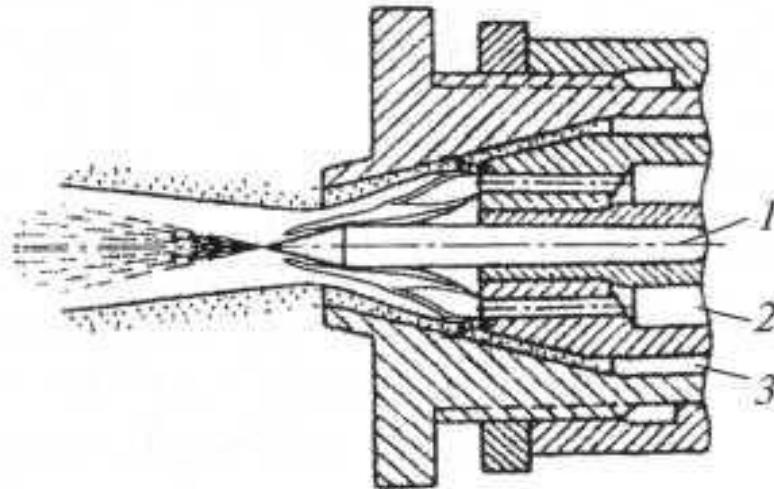
Bars 1-, 2- combustible gas (acetylene) with oxygen
